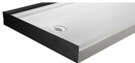
Factory-installed tile flange is 3/16" thick. Account for this thickness when planning final opening size.
