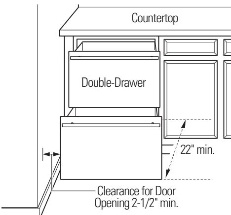
Allow 2-1/2" min. clearance between Double-Drawer and adjacent cabinet, wall or other appliances. Allow 22" min. clearance from the front for drawer opening.
