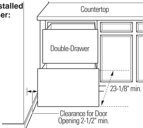
Allow 2-1/2" min. clearance between Double-Drawer and adjacent cabinet, wall or other appliances. Allow 23-1/8" min. clearance from the front for drawer opening.
