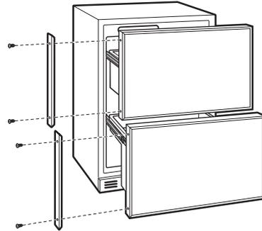
Custom handles of your choice, supplied by your cabinet maker, must be installed onto the overlay panels before they are slid into the trims. Countersink all screws into the backer panels. Screws cannot protrude from the backer panels.
