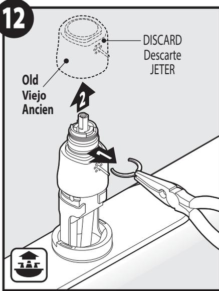
1. Using a pair of needle nose pliers, grasp retaining clip from valve body and pull out straight. Set aside.
