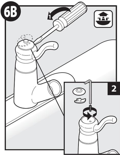
For certain models use a flathead screwdriver to pry handle cap off. Use hex wrench to remove handle screw.
