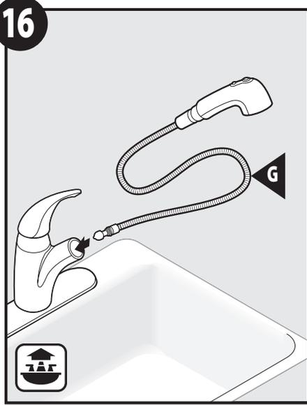
Install new Spray Wand Hose Assembly (G) through spout opening. Feed through until spray wand is fully seated.
