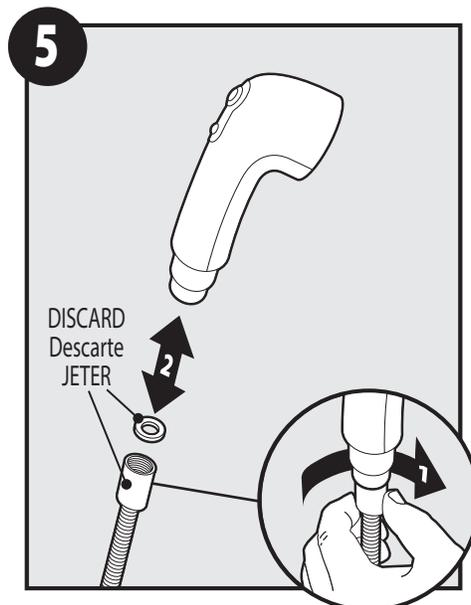
1. Unthread spray wand from hose. Set spray wand aside for re-installation.
