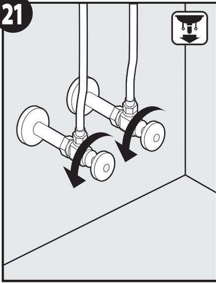
Turn water back on. Check for leaks.
