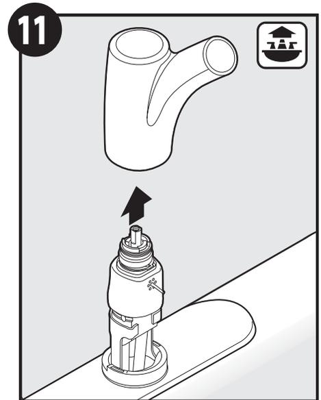
Remove faucet body shelf from valve body. Set aside for reinstallation.
