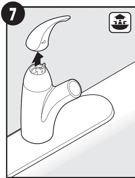
Once handle screw is removed, remove handle by pulling straight up. Set aside for reinstallation.
