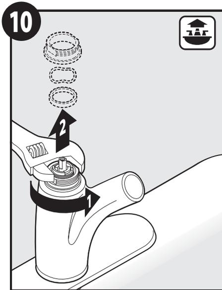
Using an adjustable wrench, remove cartridge nut, O-ring and gasket.
