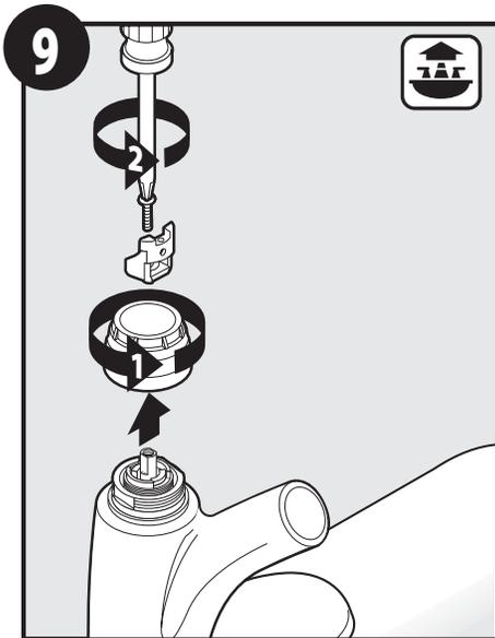
1. Loosen and remove handle dome nut from valve body.
