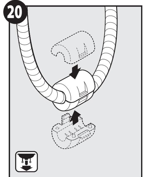
Re-attach hose weight to spray hose. Ensure hose weight snaps together.
