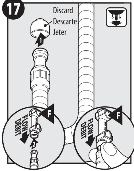
1. Remove and discard protective cap from end of spray hose.
