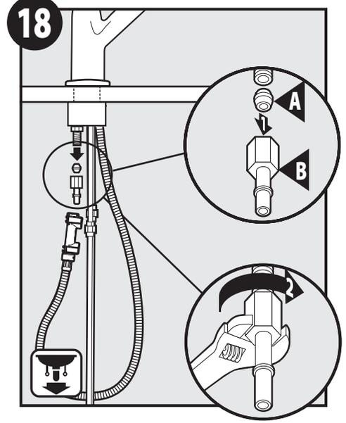
1. Install Ferrule (A) into Hose Adapter (B).
