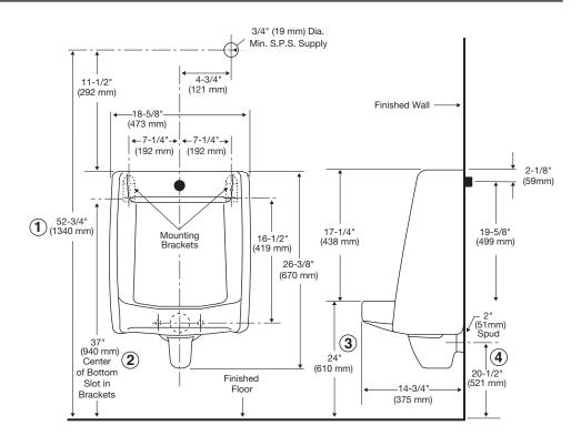
NOTE: Outlet connection 2" female threads - protrude 1/2" past the urinal.
