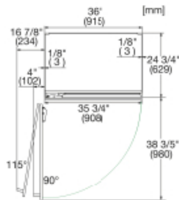
KF2902SF, KF2912SF, KF2901SF, KF2911SF, MasterCool, top view, doorway, installation drawings (US, CA)
