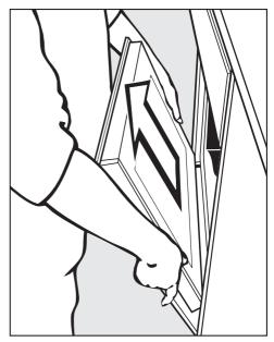
Hold the door on either side and pull it upwards off the hinge retainers. Make sure that the door is straight.
