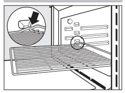
■ To remove the wire rack, lift it upwards slightly at the front when the safety notches connect with the sides of the oven.
