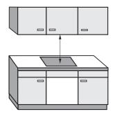
The safety distance specified by the manufacturer of the ventilation hood must be maintained between the Pro-Line element and the ventilation hood above it. If the ventilation hood manufacturer's instructions are not available or if combustible objects are installed above the ProLine element (e.g., cabinets, utensil rail), a minimum safety distance of at least 29 15/16" (760 mm) must be maintained.
