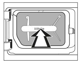
2 Then press on the handle until the lint filter is secured in position.
