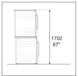
A stacking kit\* is required. This must be installed by a service technician authorized by Miele.
