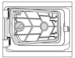
① Use the handle on the right to slide the filter insert <u>at an angle</u> behind the edge.
