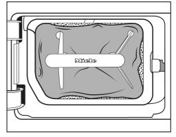
The edges of the filter do not sit properly and the filter is deformed. Lint will blow into the heat exchanger unfiltered through edges that do not sit properly. This will cause a permanent obstruction in the heat exchanger.
