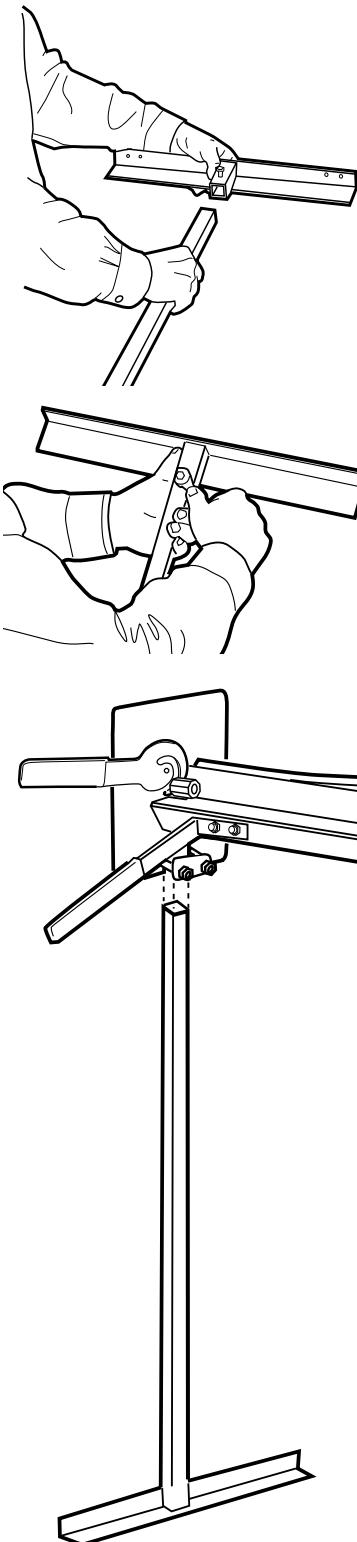
1. Insert leg shaft into leg base and tighten lock bolt to secure.
