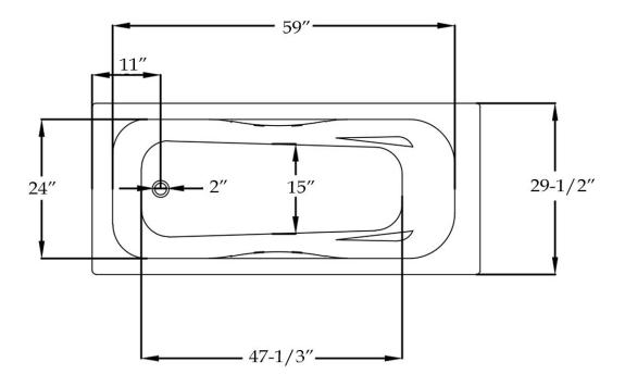
Weight (empty): 251 lbs Weight (filled): 614 lbs Capacity: 44 gal Water depth: 13-4/5"
