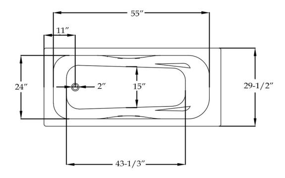
Weight (empty): 227 lbs Weight (filled): 546 lbs Capacity: 41 gal Water depth: 13-4/5"
