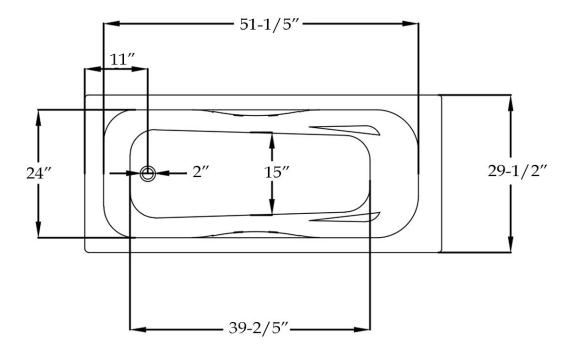
Weight (empty): 200 lbs Weight (filled): 519 lbs Capacity: 38 gal Water depth: 13-4/5"
