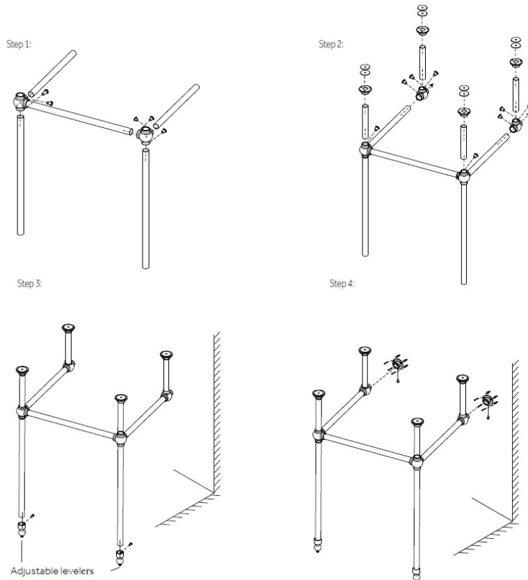
2. Once assembled, place the sink stand against the wall and in line with wall studs or wood blocking. Make sure the stand is level. If needed, adjust the small screws under each leg to level.
