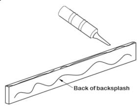
Apply a few thin beads of sealant (not included) to unpolished back and bottom edge of backsplash. Make sure all surfaces are dry.
