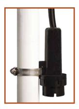
The compact level sensor detects the liquid level in the tank and sends a signal to the IP panel which displays this level in inches or centimeters for easier monitoring of the system. Pump activation and alarm levels can be adjusted using the panel touchpad - eliminating the need to go into the tank for manual adjustment.
