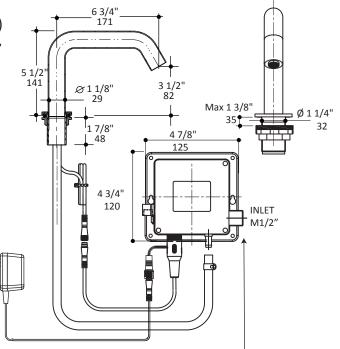
IMPORTANT: Install provided flow reducer on the water inlet
