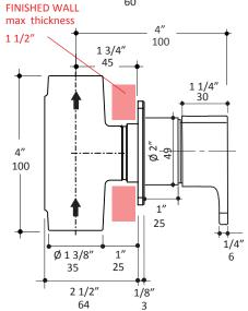
LACAVA reserves the right to revise any dimension or information on this sheet without notice. Dimensions are nominal and may vary within an industry accepted tolerance of 1/4". Drawings provided herein are meant to give the user an idea of the product and are not made to scale. Location of plumbing is meant for reference, your specific application may vary.
