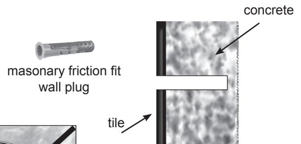
masonry friction fit wall plug
