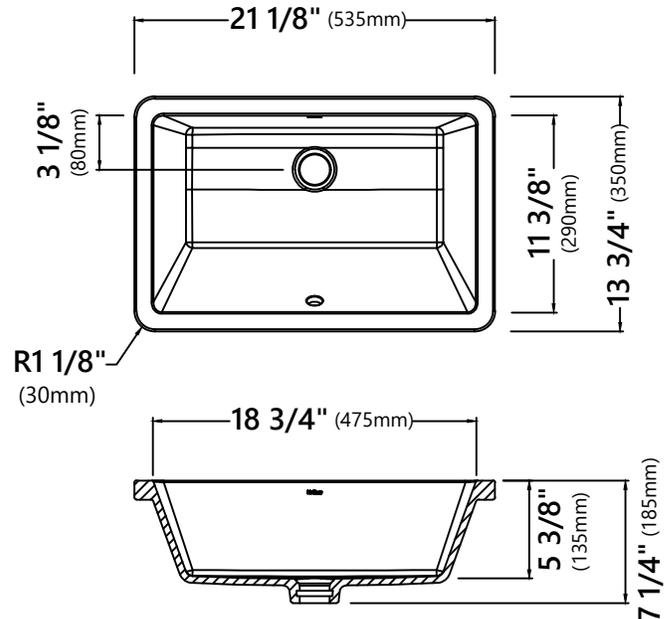
**NOTE:** Each sink may have a 3% dimension tolerance. Please measure the sink prior to installation.
