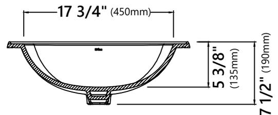
**NOTE:** Each sink may have a 3% dimension tolerance. Please measure the sink prior to installation.
