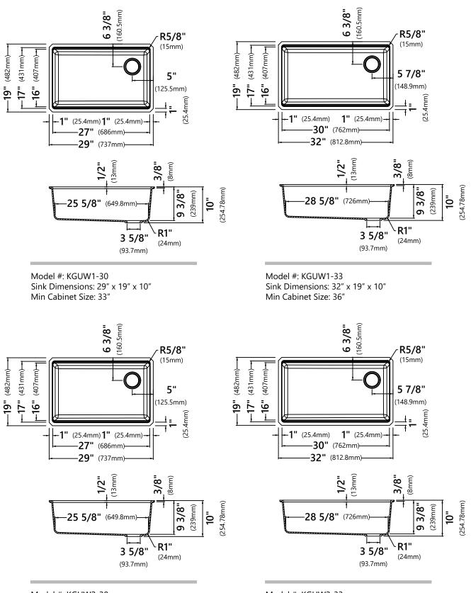
Model #: KGUW2-30 Sink Dimensions: 29" x 19" x 10" Min Cabinet Size: 33" Model #: KGUW2-33 Sink Dimensions: 32" x 19" x 10" Min Cabinet Size: 36" • Use scissors to cut along the line of the paper template for your desired reveal type (Negative, Positive, or Flushed Reveal)
