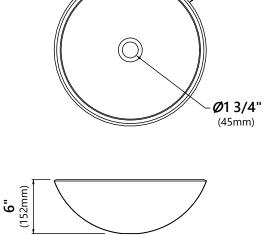
Model #: GV-101-19mm, GV-391-19mm, GV-398-19mm, GV-399-19mm, GV-680-19mm Sink Dimensions: Ø17" x 6" Glass Thickness: 19mm
