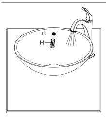
After installing faucet, remove aerator (G) with included aerator key (H). Turn water on for 30 seconds to remove any debris. Reassemble aerator (G).
