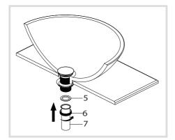
Slide the nut (6) over the tail pipe (7). Place the washer (5) into the nut and tighten. Do not overtighten.
