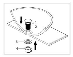
Place the washer (1) underneath the flange of the pop-up body (2). Slide the pop-up body (2) down through the drain hole on the vessel or basin. From underside, slide the washer (3) against the bottom of the vessel or basin, thread on the coupling nut (4) and tighten. Do not overtighten.
