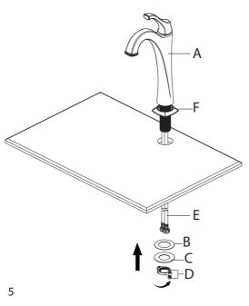
Before installation, ensure that the flange (F) is placed on the bottom of the faucet assembly (A). Place faucet (A) through the 1-3/8" holes in countertop . Secure the faucet (A) to the countertop using the plastic washer (B), metal washer (C) and nut & screws (D) provided. Hand tighten the nut onto the end valve shank. Lock the nut into position by tightening the screws (D) with a phillips screwdriver.
