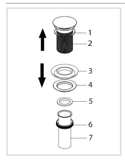
Unscrew the nut (6) from the pop-up body (2), move over the tail pipe (7) and washer (5), then unscrew the coupling nut (4) and remove the washer (3).
