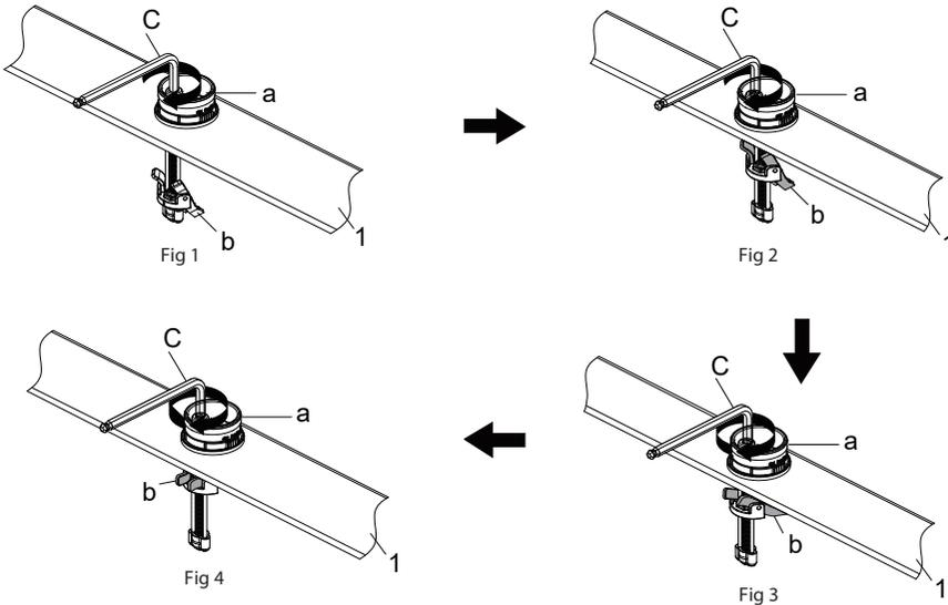
Press the base (a) so that it can not move, then turn the screw with the provided hex wrench (C, HEX: 6.0mm) clockwise, as shown Fig 1. When the mounting plates (b) make contact with the sink (1), continue to turn the screw with the provided hex wrench (C, HEX: 6.0mm) clockwise, as shown Fig 2, until the base (a) is completely tightened and secured, as shown Fig.4.
