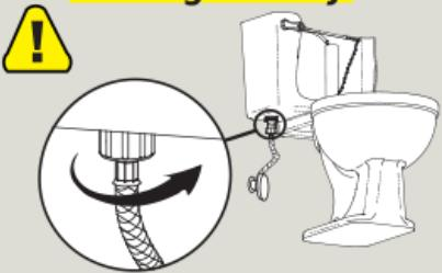
b) Turn on water supply. Let tank fill completely.
