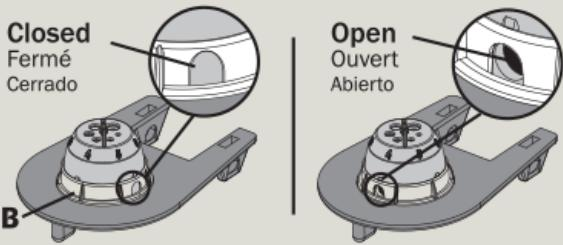
b) Rotate dial (D) to align next lowest number with arrow (A). Repeat process in steps 5b & 5c and adjust dial until setting allows water to drop within 1/2" of pencil mark.
