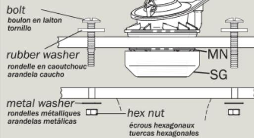
Tank will wobble initially. Apply downward pressure to tank with hand to keep tank level. Alternate tightening each hex nut until tank is stable & level. Use adjustable wrench to tighten hex nuts if needed. Do not continue tightening if tank & bowl touch. Do not overtighten as the tank may crack.
