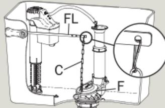
**5** a) Reconnect water supply. Do not use sealant / tape. **Hand tighten only.**
