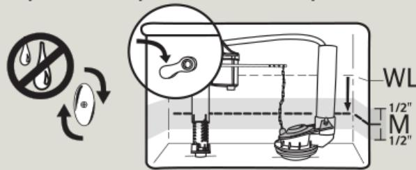
**6** a) Rotate hole in band (B) to open position. Repeat process in steps 5b & 5c before proceeding to step 6b.
