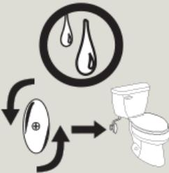
c) Turn off water. Flush. If water level (WL) drops within 1/2" of pencil mark (M), flapper install complete. If not, proceed to next step.
