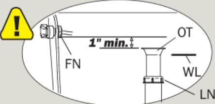
b) Attach to overflow tube with S-clip. Trim tube if kink occurs.
