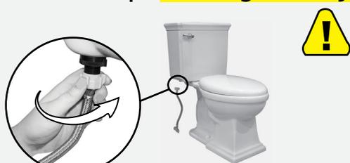
Note: We recommend replacing with a flexible supply line (pictured)
