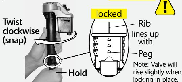
b) Place locked valve in tank as shown.
