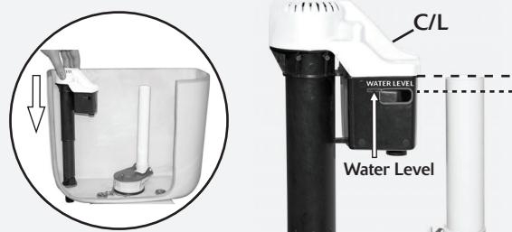
\*Note: This positions critical level (C/L) on cover 1 inch above overflow level. (Code Requirement)
