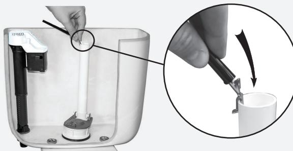
c) Attach other end of tube to fill valve. If tube kinks or is too long, trim prior to attaching.
