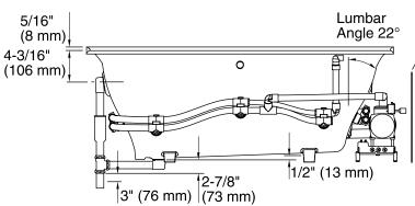
Pump/Control Access 34" (864 mm) x 15" (381 mm)
