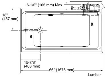
No change in measurements if connected with drain illustrated. (K-7147-AF)
