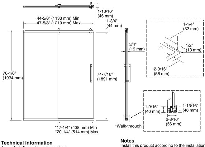
All product dimensions are nominal. Base-To-Wall 1/2" (13 mm) Radius – Max: Shower Ledge Min 2-3/16" (56 mm) Flat: Shower Wall Min 1" (25 mm) Flat: Install this product according to the installation guide.
