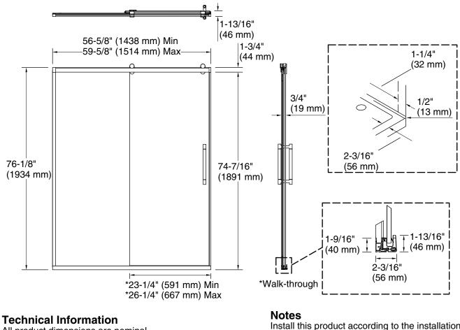
All product dimensions are nominal. Base-To-Wall 1/2" (13 mm) Radius – Max: Shower Ledge Min 2-3/16" (56 mm) Flat: Shower Wall Min 1-1/4" (32 mm) Flat: Install this product according to the installation guide.
