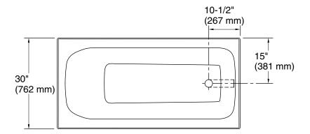
No change in measurements if connected with drain illustrated. (1381626)
