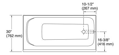
No change in measurements if connected with drain illustrated. (1381626)
