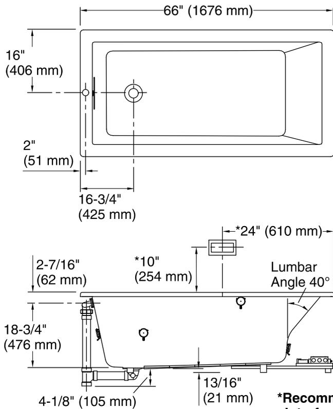
No change in measurement if connected with drain illustrated. (K-7272)
