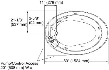
No change in measurements if connected with drain illustrated. (K-7166-AF)
