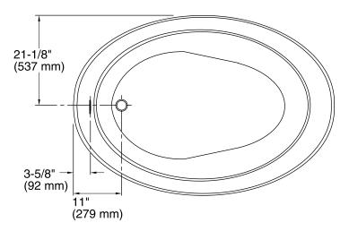
No change in measurements if connected with drain illustrated. (K-7161-AF)
