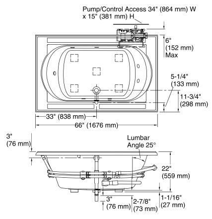
No change in measurements if connected with drain illustrated. (K-7161-AF)
