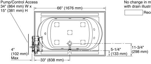
No change in measurements if connected with drain illustrated. (K-7161-AF)
