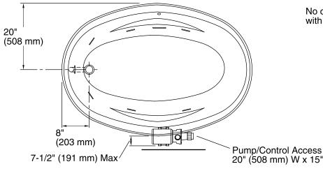
No change in measurements if connected with the drain illustrated. (K-11677)
