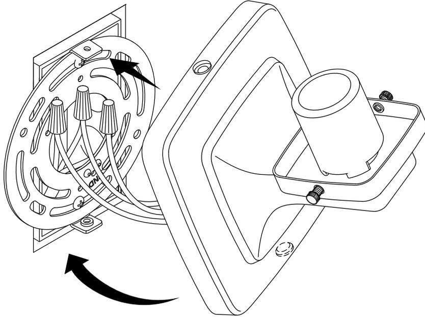
**NOTE:** As you are positioning the sconce body onto the sconce mounting plate, carefully tuck the wiring into the outlet box.
