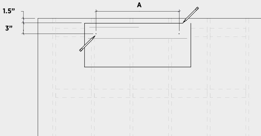
3. Screw two (2) screws at the marked points, leaving a slight gap between the screw head and the wall. Use only screws that are suitable for your wall material (these screws are not included).
