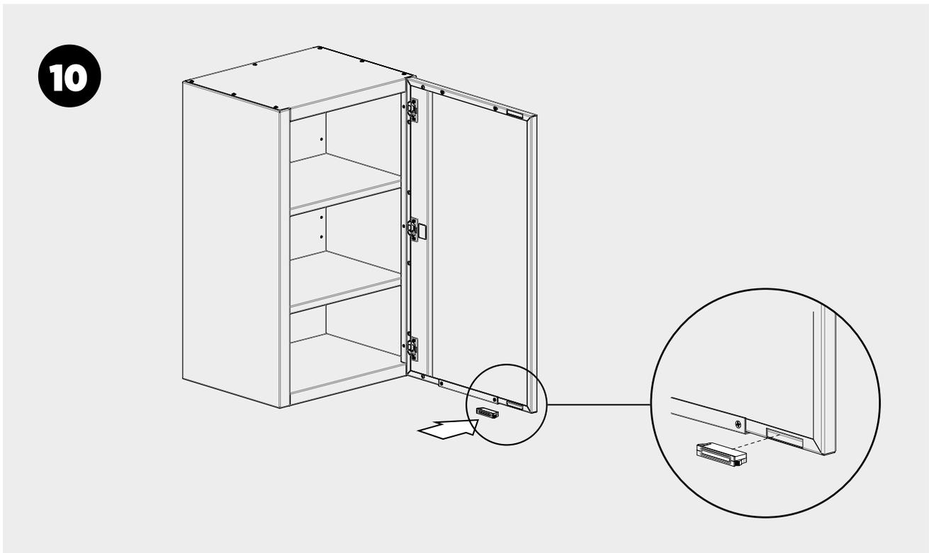
11. Remove the film from the magnet plate and place it on the post. The corner should be on the L-shaped engraving.
