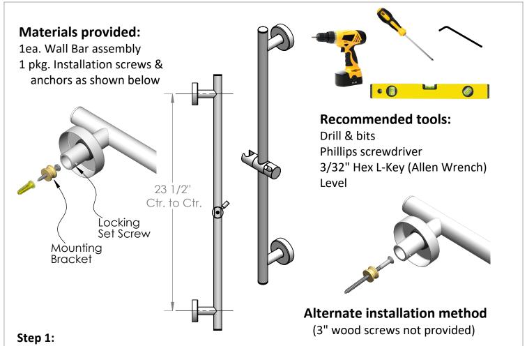
Determine appropriate mounting location, and mark the mounting centers. For the alternate installation method, locate suitable in-wall structural framing (2X4 studs or cross-members).
