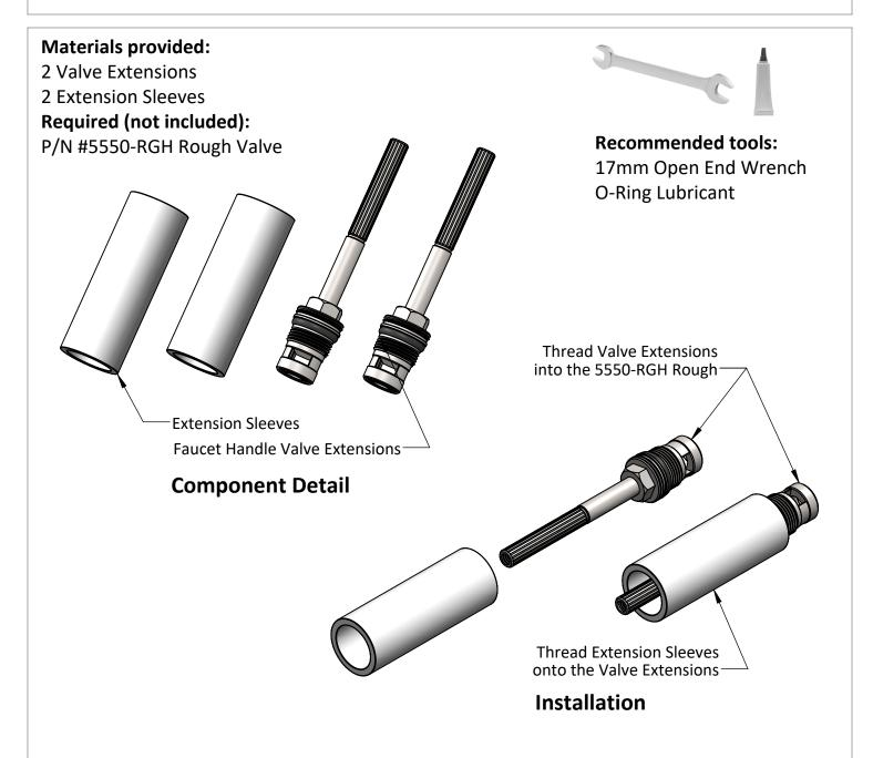
**Step 1:** Apply suitable lubricant to the Faucet Handle Valve Extension O-rings.
