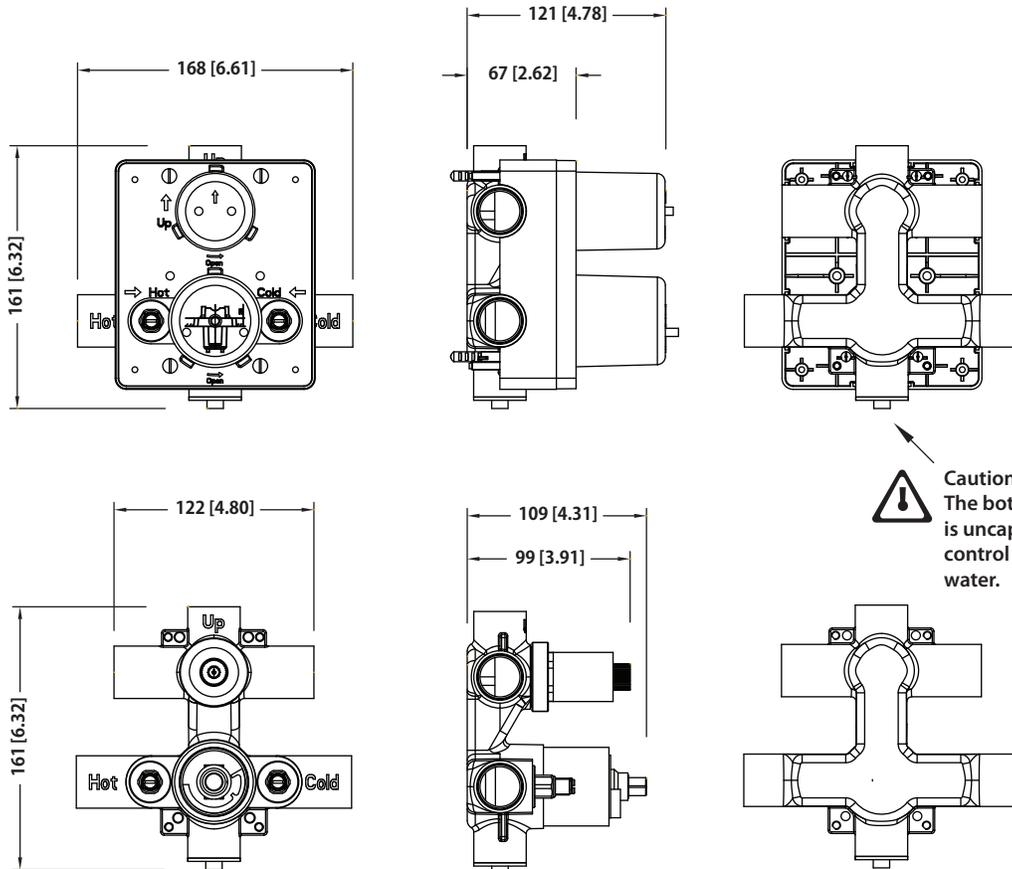
**TVL.2750 | 3/4" Thermostatic Valve With 3-Way Diverter And Integrated Volume Control** Page 2 of 2
