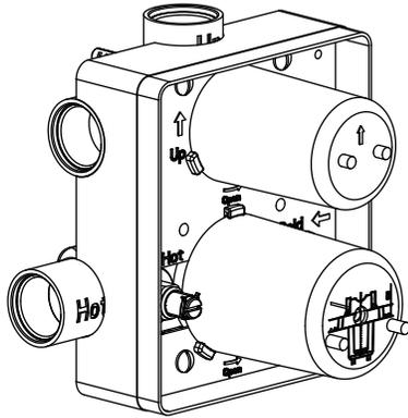
**!** A separate volume control is **not** needed to turn water supply off. Volume control functionality is integrated within this valve.
