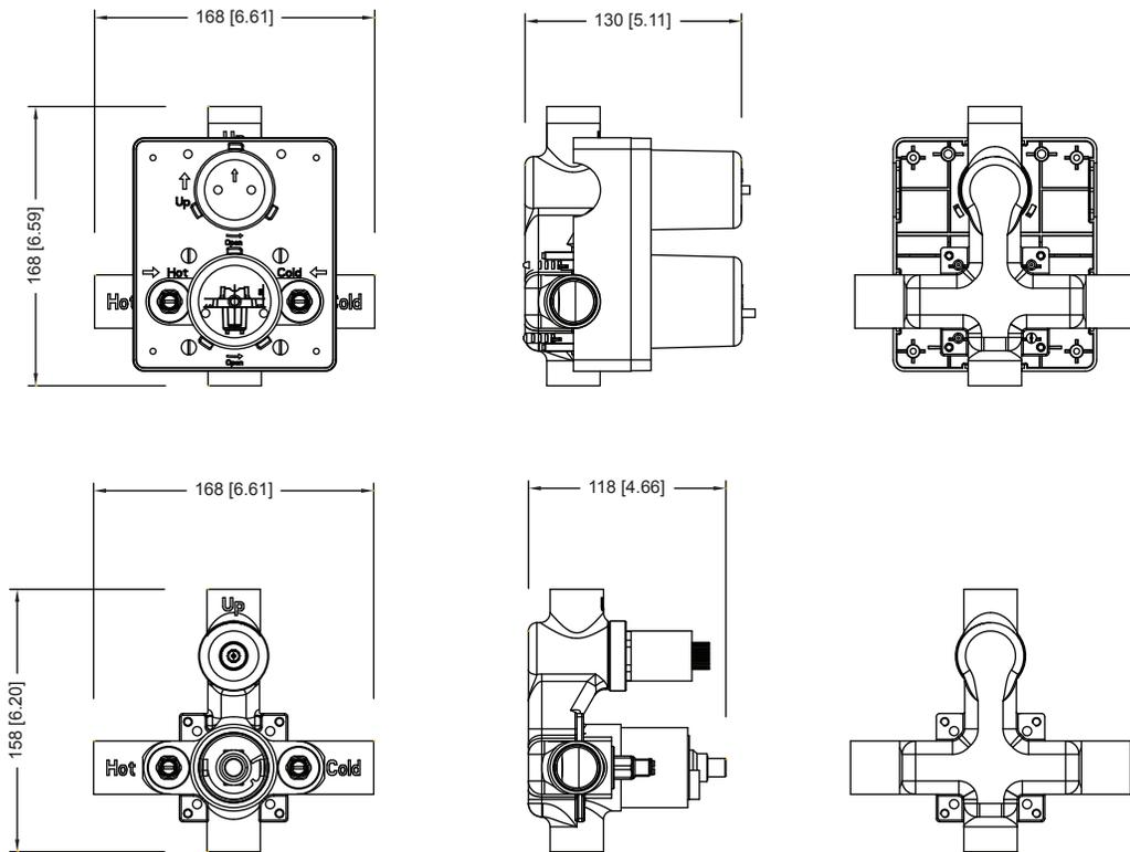
TVL.2700 | 3/4" Thermostatic Valve With 2-Way Diverter And Integrated Volume Control
