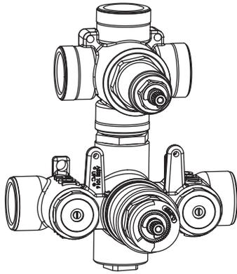
**!** A separate volume control is **not** needed to turn water supply off. Volume control functionality is integrated within this valve.
