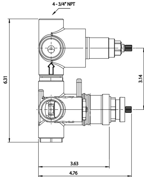
TVH.4301 | 3/4" Thermostatic Valve With 3-Way Diverter & Integrated
