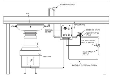
**NOTE:** The MRS control center should be mounted 1-1/2" (38.1 mm) back from the front surface of the table.
