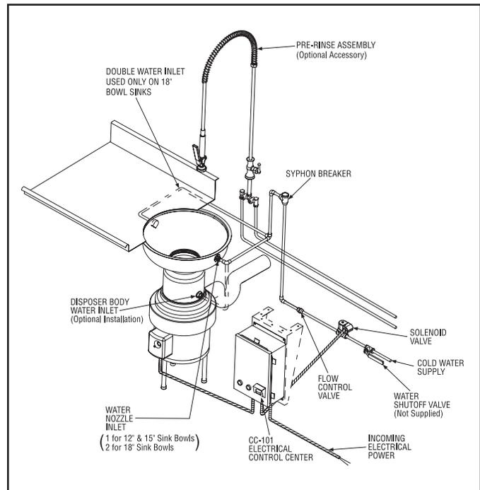
Figure 2. Typical Installation Diagram
